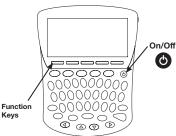
On/Off: Turns the unit on and off. Function Kevs: Each of these unlabelled keys corresponds to the function that appears directly above it on the screen.
