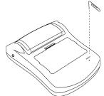
Warning! Pressing the reset button with more than light pressure may permanently disable your device. In addition, resetting the device erases settings and information entered in its built-in book and in an installed book card.
